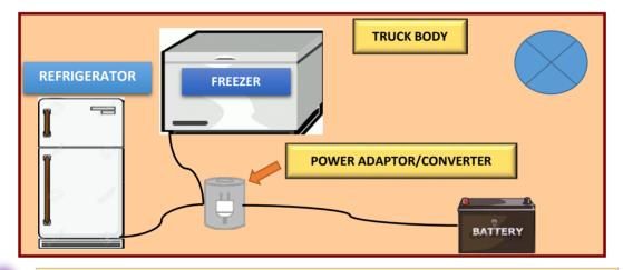
A LAYOUT OF THE MOBILE UNIT INDICATING THE LOCATION OF ALL EQUIPMENT MUST BE SUBMITTED TO THE LOCAL HEALTH DEPARTMENT. PLEASE REFER TO THE DIAGRAM ABOVE TO ASSIST IN PREPARING A PROPER UNIT LAYOUT.
